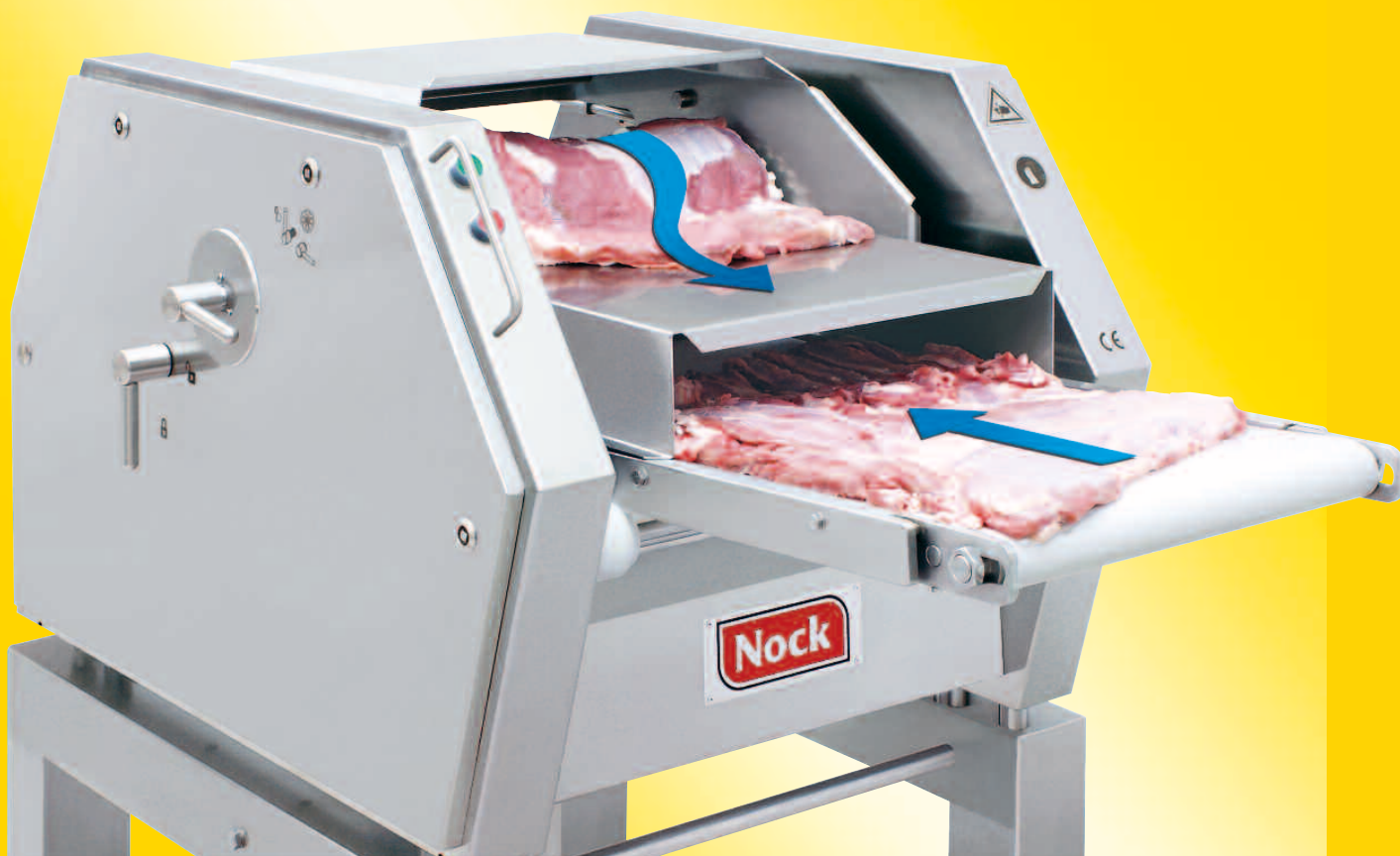
Breast of veal on a Doner cutting machine Cortex CB 503 KEBAB with NOCK Integrated Product Return System®
