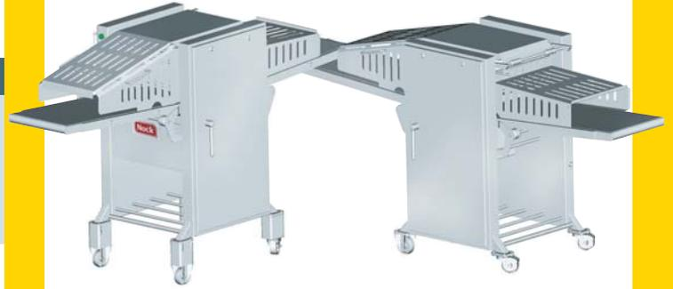
Cubes e.g. from poultry breast can be cut in a second operation or with two machines standing at a 90° angle. The meat passes automatically onto the second machine and needs no second operator.
