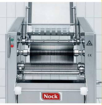
Cortex CB 495/5K SLICER after removing the conveyor belts
