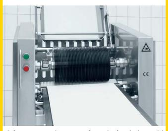
Saftey cover opened, transport roller made of synthetic material with stainless steel core (optional)
