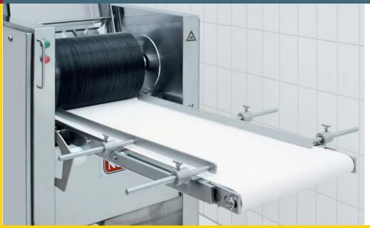
Adjustable lateral guides at infeed conveyor belt
