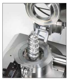
Vertical cutting housing with single cutter set
