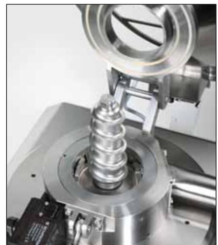
Vertical cutting housing with single cutter set
