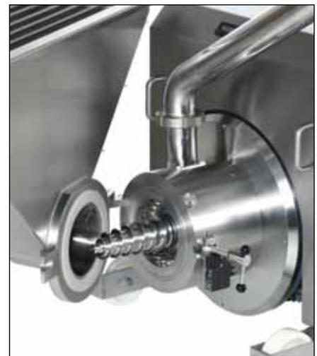
Horizontal cutting housing with double cutter set
