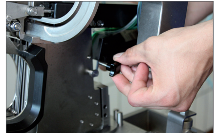
Service-friendly: knife replacement without tools
